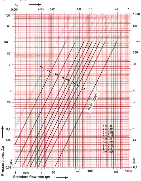
The curves "1-9" apply to the nominal lift (2 K) of the valve cone.
